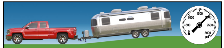
FIGURE L4: Truck and trailer angled up (higher pressure)
