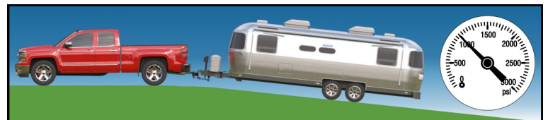
FIGURE L5: Truck and trailer angled down (lower pressure)
